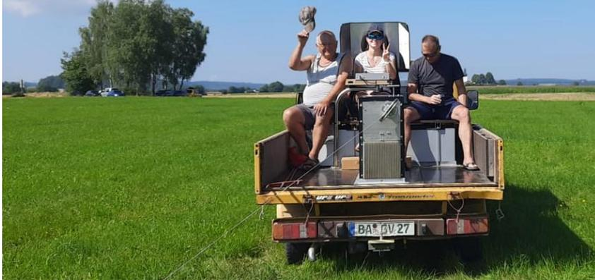
Hohenpözl: Heiligenstadt, Bamberger Gleitschirmclub, a series module on VW flatbed for mobile/stationary towing since February 2021. 16kWh battery.
